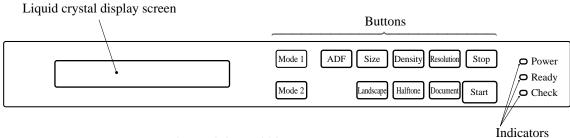
Figure 2.3 M3097E+ operator panel
